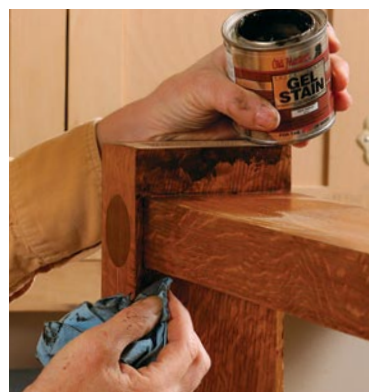
Imitate dirt buildup. Gel stain, applied with a rag and allowed to set 10 minutes, ages the finish easily.
